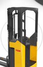
SSO SIT-ON STACKER **LIFT CAPACITY** 1600/2000 kg LIFT HEIGHT Up to 7 metres
